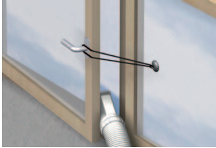
Fig. 4 Exhaust air with open window
